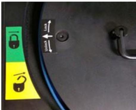
The figure above shows labels that indicate if the sample plate cover is in the locked or unlocked position. Here, it is shown in the locked position. The Bullet Blender will not start until the
