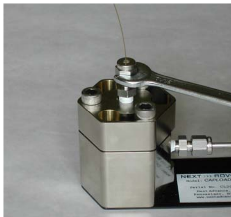
Use a wrench to tighten the nut, forcing the ferrule to squeeze tightly around the capillary.
