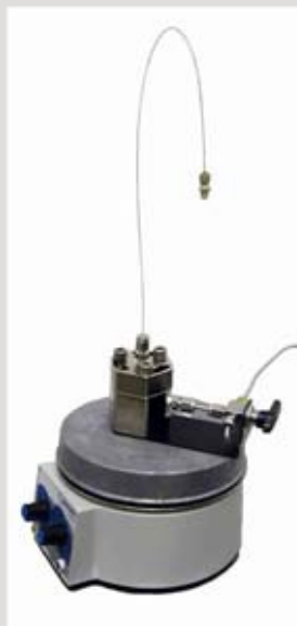
Pressurized gas forces the sample liquid into the capillary.
