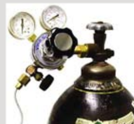
Pressurized gas forces the sample liquid into the capillary.
