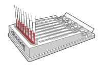
**STEP 3 > FLIP IT** Flip up well tab with finger or robot
