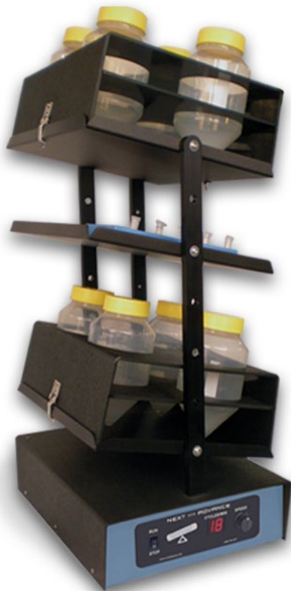
The Infinity Rocker Stack-3 with two Stabilizer™ container racks
