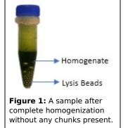
4. Remove the tubes and visually inspect the samples to confirm complete homogenization (Figure 1). **Note:** If unhomogenized tissue is seen, homogenize for additional 30 seconds.
