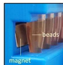
Figure 2: Magnetic beads separate to the back wall of the tubes, when placed in the magnetic rack.
