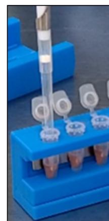
Figure 3: Using pipette tips, carefully remove the supernatant. If needed, hold the tube to prevent the tube from moving/spinning.
