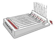
Using light force, flip up the 8-well tab with your finger or pipette tips to fully vertical.
