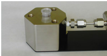
The sample tube protrudes from the base for easy insertion and removal.
