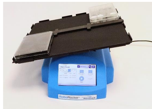
A RoboRocker with a culture plate on the platform. The platform can hold up to 6 culture plates, tilting them to a precise angle so that the culture medium flows past the cells at the desired rate.
