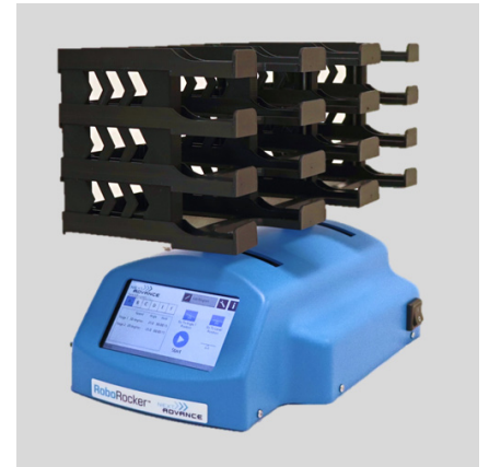
The rack on this RoboRocker securely holds up to 12 culture plates while allowing plenty of aeration.
