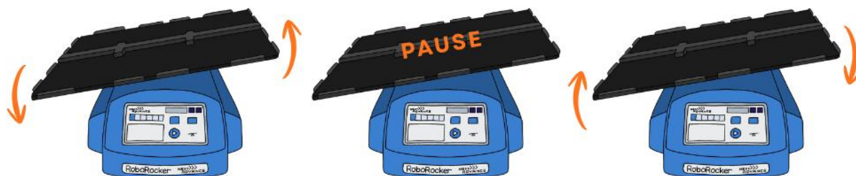
Figure 3. The RoboRocker tilts to the desired angle (left), then holds that angle for a defined pause period (center), enabling full perfusion of fresh medium and complete waste removal. After the pause, it advances to the next angle (right). In contrast, traditional rockers only allow short periods of perfusion and recirculate the same portion of the medium, leading to nutrient depletion and waste buildup.
