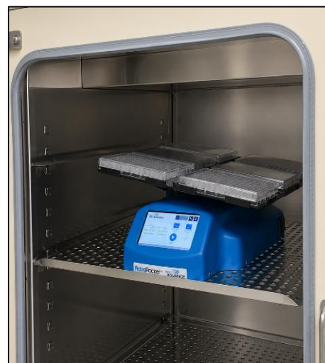
Figure 1. A RoboRocker operating inside an incubator.
