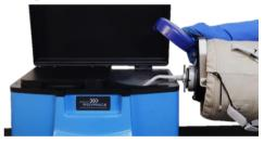
NEVER pour the liquid nitrogen into the dry ice insert. Follow standard laboratory safety precautions while handling liquid nitrogen. Make sure that the compartment cap is properly seated.
