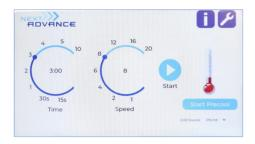
We recommend pre-cooling the instrument to maintain the sample temperature and therefore its integrity during the entire homogenization procedure. Pre-cooling the instrument ensures the chamber achieves 4°C before adding temperature sensitive Once the chamber samples. sufficiently cooled, the Bullet Blender will indicate "PRECOOL COMPLETE" and the thermometer will turn blue. The instrument is now ready to run your samples.
