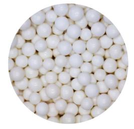
RNase-free zirconium oxide beads (ZROB10-RNA) undergo a special cleaning process. They are guaranteed and certified to be RNase-free.
